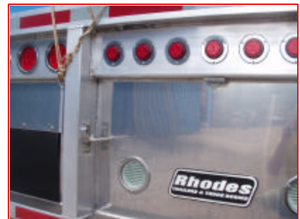
? Steps, lights, closure plate
