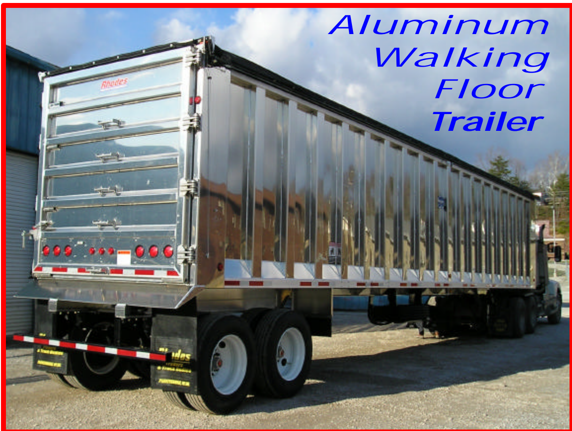
AWF48-8-102-2 All-Aluminum Walking Floor T trailer
